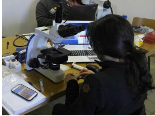
Fig. 2: Workplace with a full ISAS system created by Proiser R+D. The CASA system was composed by UB203i phase contrast microscope, video camera of 500 fps, counting chambers (Spermtrack® 10 and 20 \mu\text{L} ) and a computer with ISAS software.
