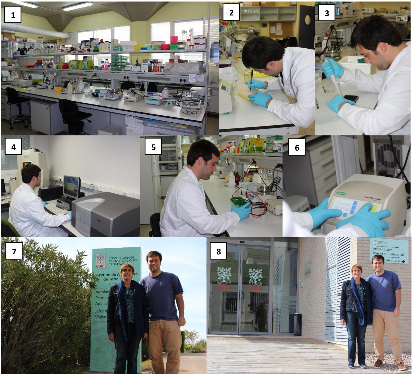
Figure 1 – Main Laboratory; Figure 2 – Preparing samples; Figure 3 – Using a black multiwell plate for DNA analyses; Figure 4 – Reading DNA fluorescence using a spectrophotometer; Figure 5 – Electrophoresis (Western blot); Figure 6 – Membrane transference (Western blot); Figures 7 and 8 – Doctor Inmaculada Varó and Martim Magro.
